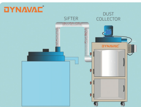
Dust particles collection from sifter during sieving operation
